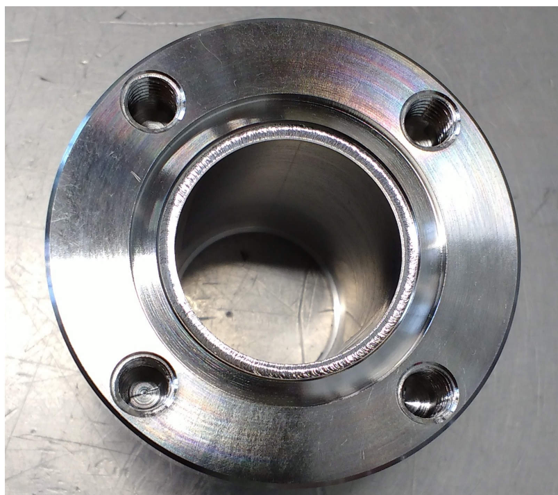
Figure 5.15: The welded joint between niobium and the titanium RF port flange.
