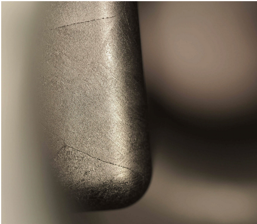
Figure 5.22: The surface appearance of the ridge after the 120 \mu\text{m} etch.
