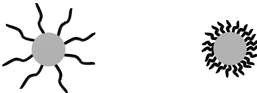
Chart 4.1. F127 micelle (left) and P104 micelle (right). PEO corona shells are shown in black.
