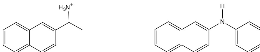
Scheme 3.1. Chemical structures of 2-naphthyl-1-ethylammonium cation ( \text{NpH}^+ , left) and N-phenyl-2-naphthylamine (Ph-A-Np, right).
