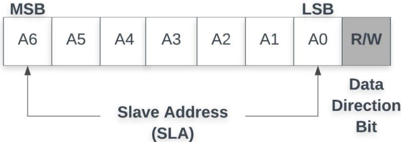
Figure 9 Format of address byte for sending the slave address [5]
