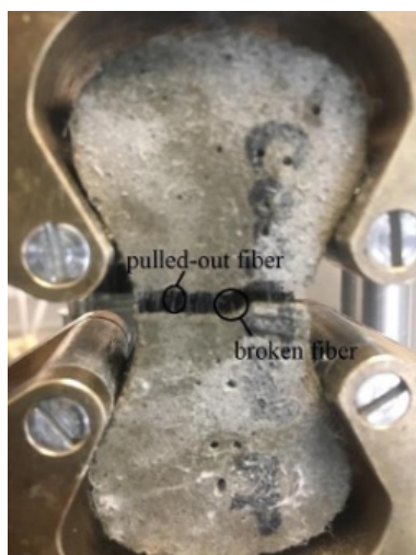
Figure 9. Coated PP-reinforced mortar under tension.
