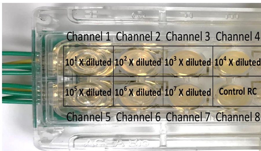
Figure 4-10. Shows the distribution layout of bacterial samples in the 8 wells of the E-plate microelectrode for the impedance testing of samples 50% stepwise dilution.
