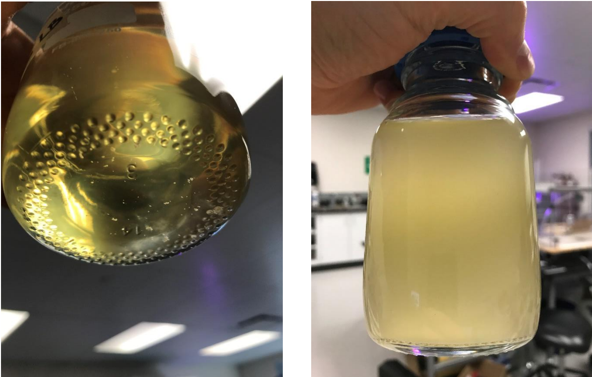
Figure E-2. Picture on the left-hand side shows clear LB broth with the bacterial cells that are just transferred to the container. Bacterial pellets can be seen at the bottom of the glass. Picture on the right-hand side shows the same growth media after one day of incubation, cloudy and saturated of bacteria.
