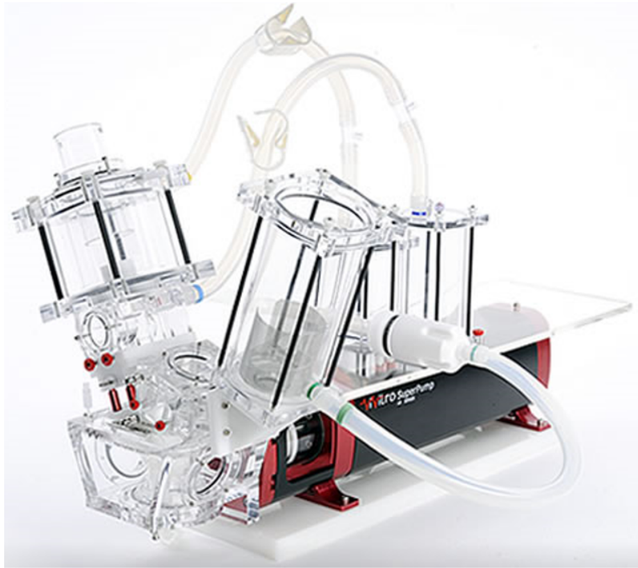
Figure 1.3: Pulse Duplicator system, ViVitro Labs Inc.[41]
