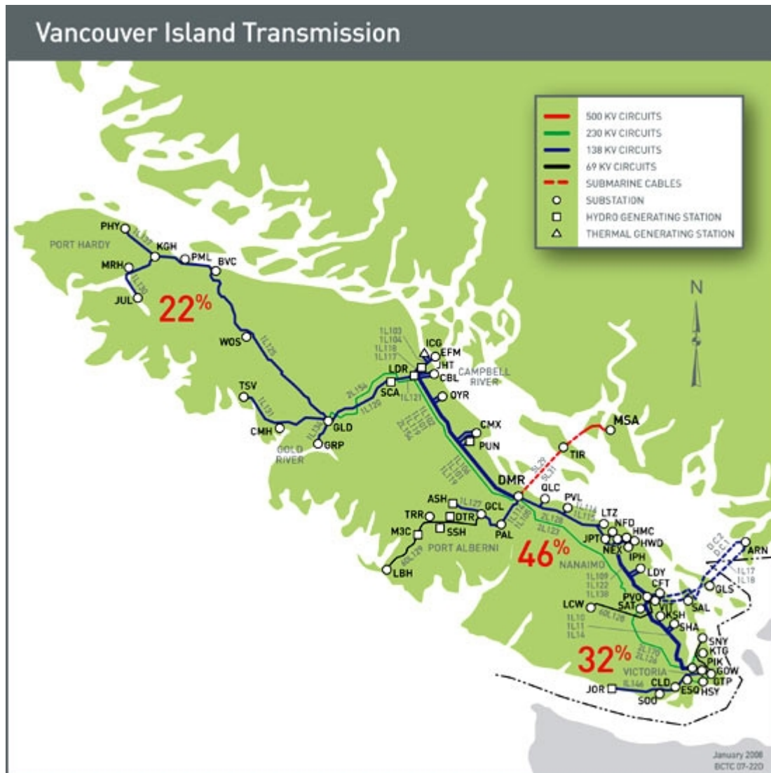
Figure 4.1: Vancouver Island Transmission and Electricity Demand Locations (Image used with permission from BC Hydro transmission website [53])
