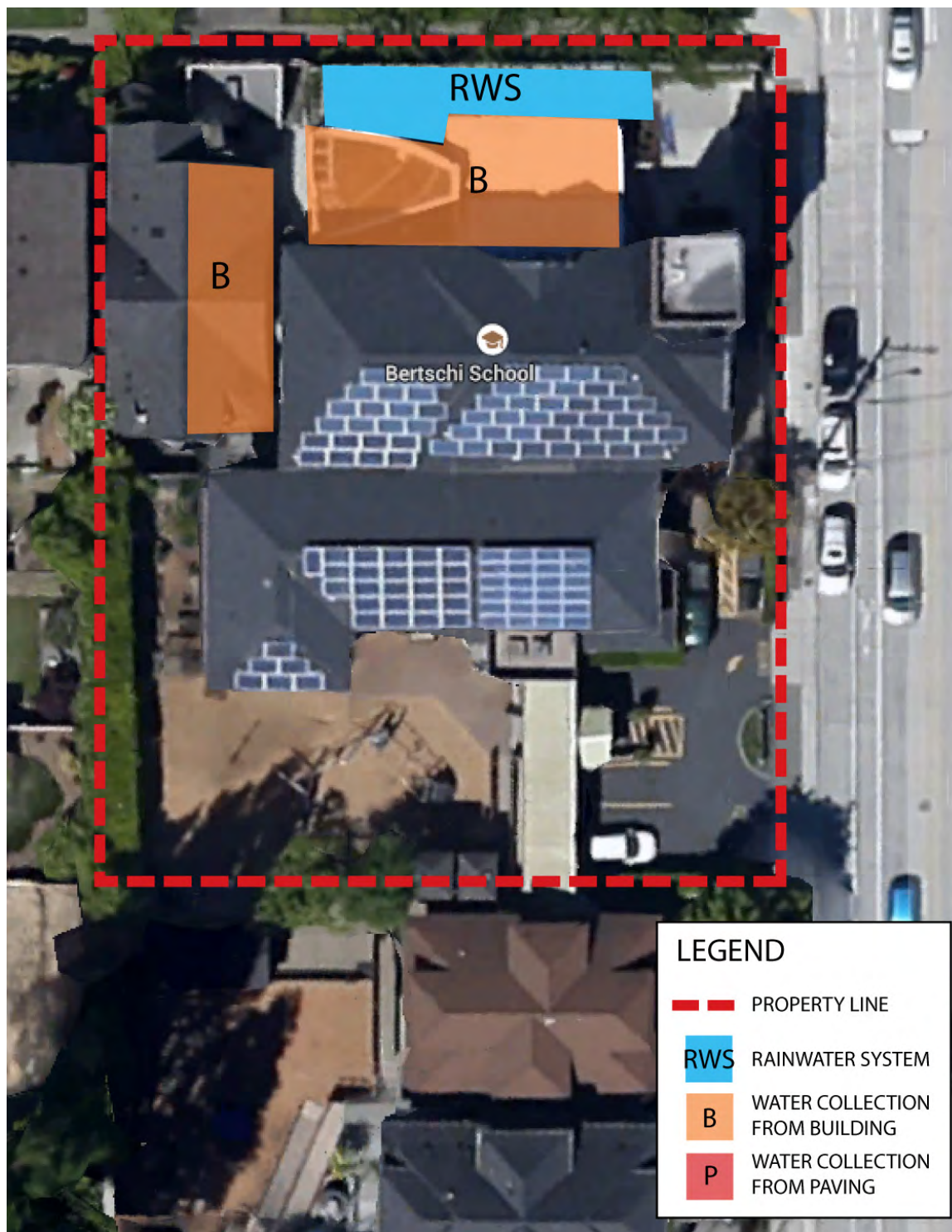
Figure 3.3: Location of Bertschi's rainwater system and water collection areas.
