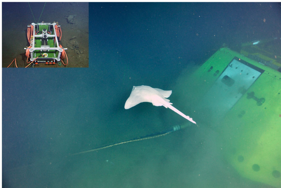
FIGURE 2 Endeavour node and typical instrument platform (inset) of the North-East Pacific Time-Series Undersea Networked Experiments cabled observatory network operated by Ocean Networks Canada
