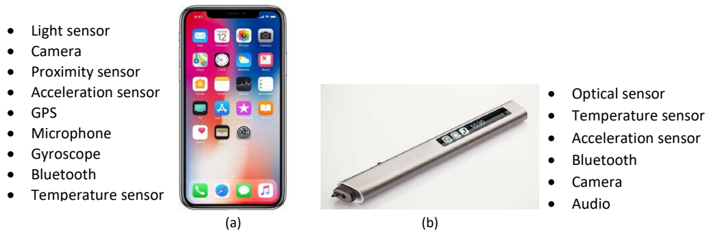
Figure 2.1: Examples of sensors on current smart mobile devices. (a) iPhone X. (b) Phree.
