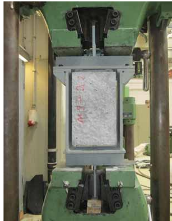
Fig. 12: Test set up for the pull-out tests.
