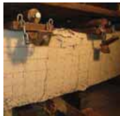
Figure 11: Typical failure mode of GG-beams
