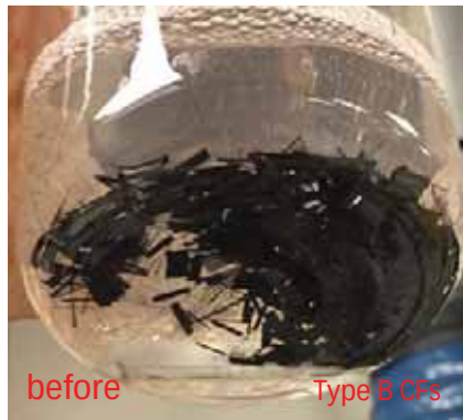
Fig 10a: Type B CFs before dispersion in MG7101
