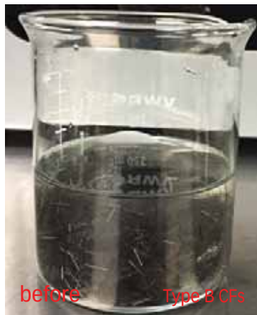
Fig 8a: Type B CFs before dispersion in solution of Methylcellulose and water
