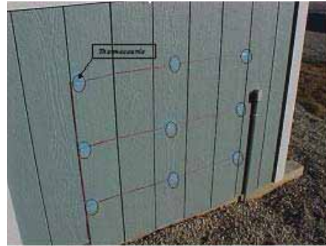
Figure 5. Exterior wall thermocouples
