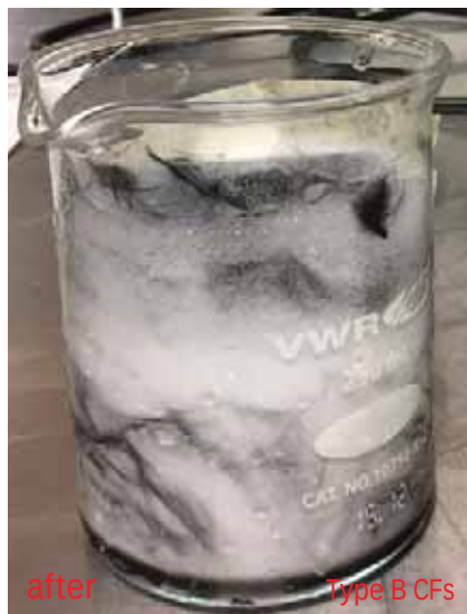
Fig 10b: Type B CFs after dispersion in MG 7101
