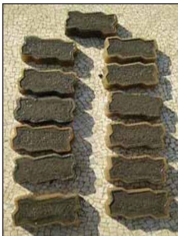
Figure 2: Alkali activated concrete paver blocks at rest period
