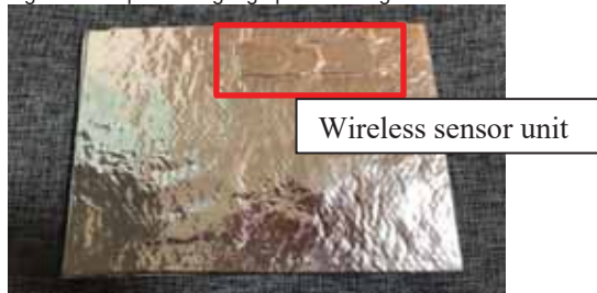
Fig. 2. Image showing the micro-pressure sensor inside a VIP
