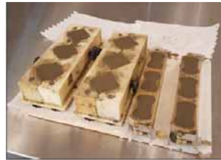
Fig 6: Mortar Mix in Cube and Briquette Molds
