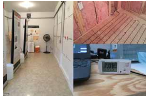
Figure 4: Interior of test hut, heated floor, and temperature control.
