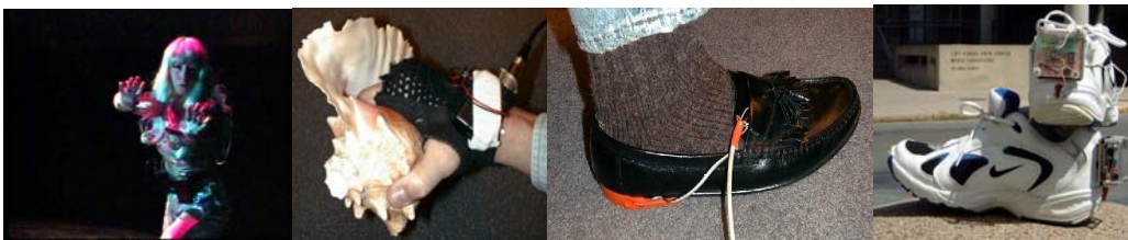
Figure 5 - Body Controllers: (left to right) Tomie Hahn as PikaPika, Cook's Pico Glove, Cook's TapShoe, Paradiso's wireless sensor shoes.
