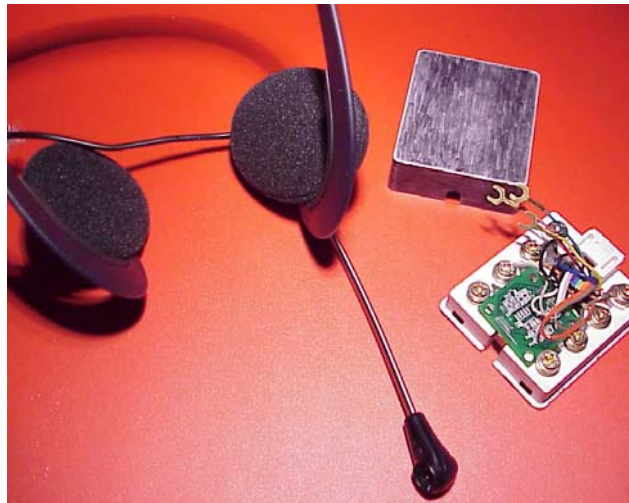
Figure 46 - Headset with accelerometer chip.
