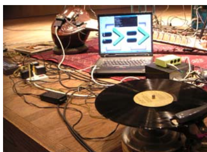
Figure 95 - ESitar Interfaced with Trimpin's Eight Robotic Turntables.
