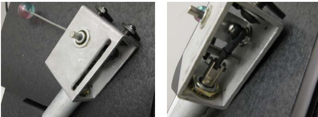
Figure 60 - Singer Hammer with added ball-joint striking mechanism.
