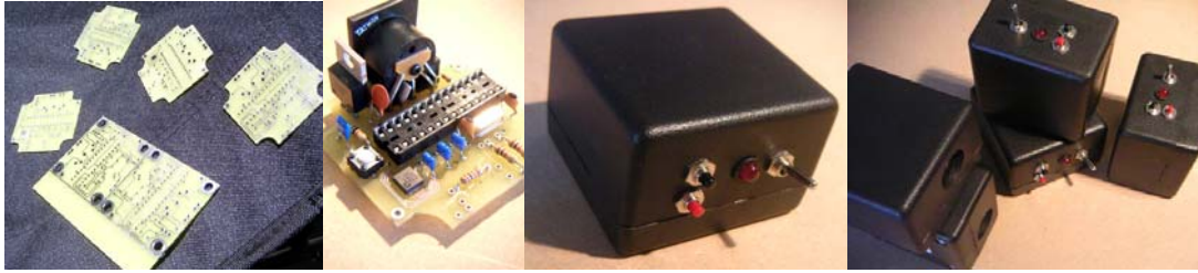
Figure 52 - The KiOm Circuit Boards and Encasement.
