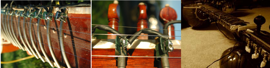
Figure 43 - The network of resistors on the frets of the ESitar 1.0 (left, middle). The ESitar 2.0 full body view (right).
