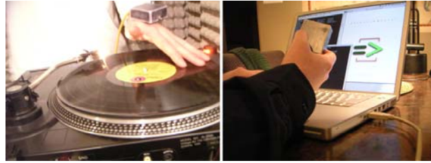
Figure 56 - Wearable sensor used to capture scratching gesture of turntablist (left). Wearable sensor used in conjunction with live Computer Music Performance using Chuck (right)..
