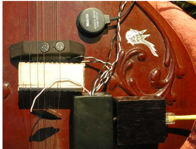
Figure 45 - Gesture capturing sensors at base of ESitar 1.0.
