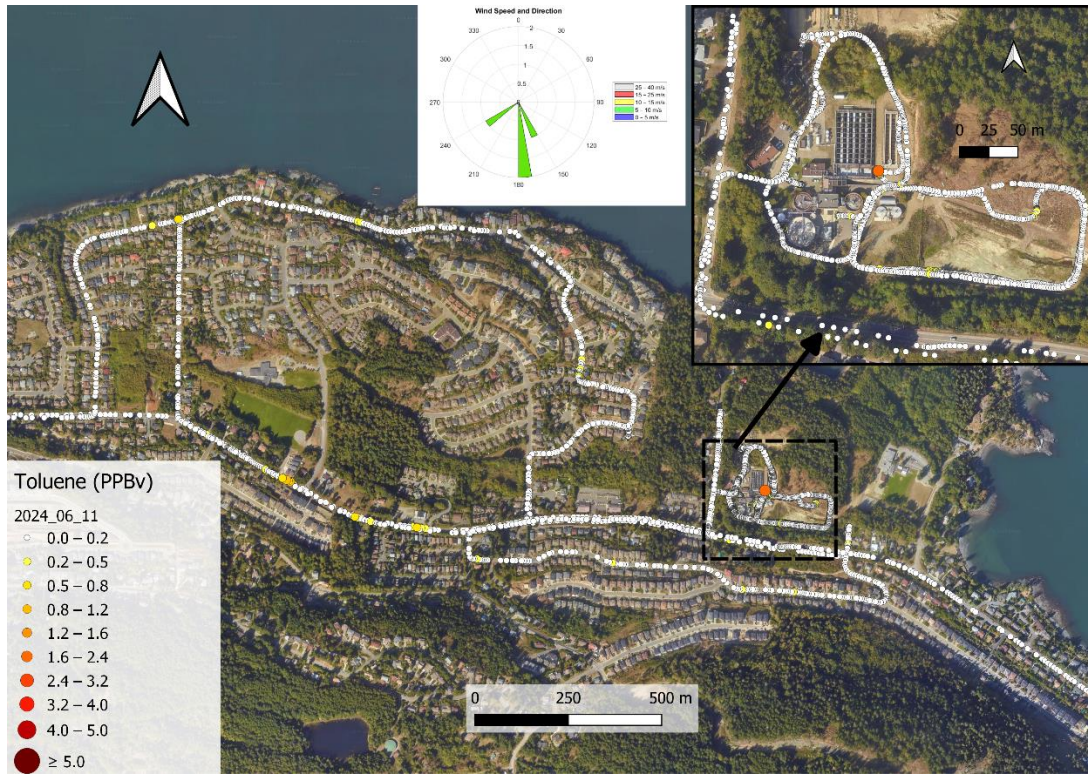
Figure 65 Toluene concentrations in the vicinity of the GNPCC on June 11, 2024.
