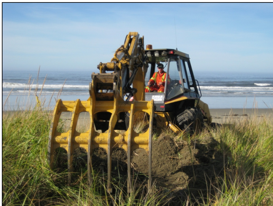
Figure 2.5. Removal of Ammophila spp. from the foredune near transect 1 on September 21, 2009. Notice the specialized bucket design (i.e., finger-like appendages to sift through sands).
