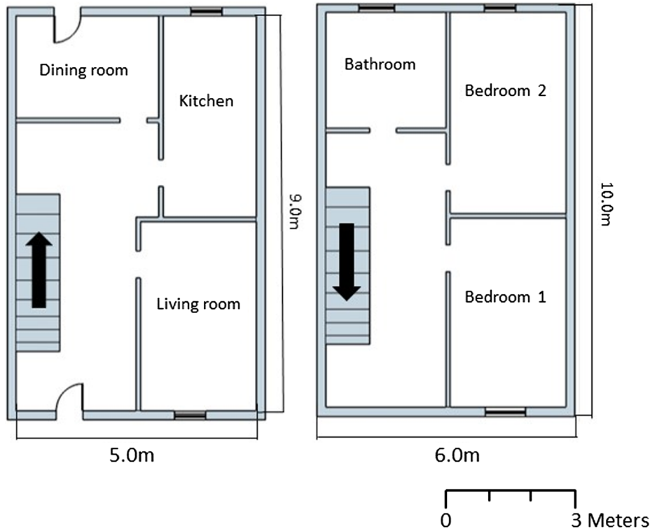
Fig. 3. Floor plan illustrating the assumed room structure of the dwelling with ground floor (left) and 1st floor (right). Approximate internal and external dimensions are shown.
