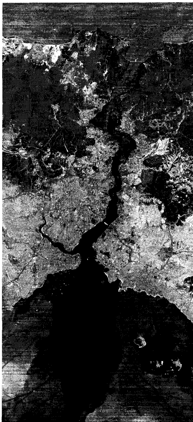
Figure 3.12.: ASTER satellite image from June 16, 2000 of the Bosphorus and its Black Sea and Sea of Marmara junction regions. Land area is shown as false colour composite of visible spectral bands with 15m spatial resolution. The water area image is derived from infrared bands with 90m resolution. Colour represents surface temperature with darker colours indicating colder waters. The scene is an extended version of that shown in figure 2.4.
