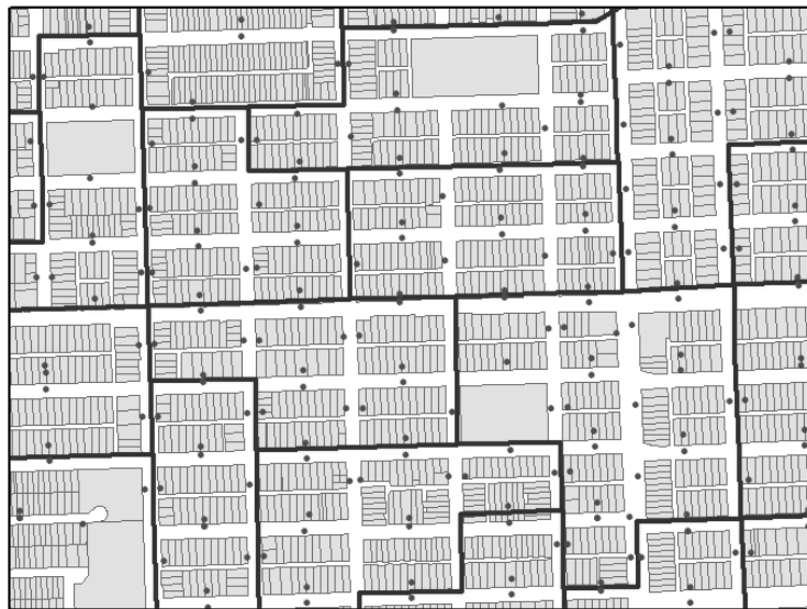
Figure 55. Spatial resolution of cadastral data, six digit postal codes and dissemination areas in Vancouver.
