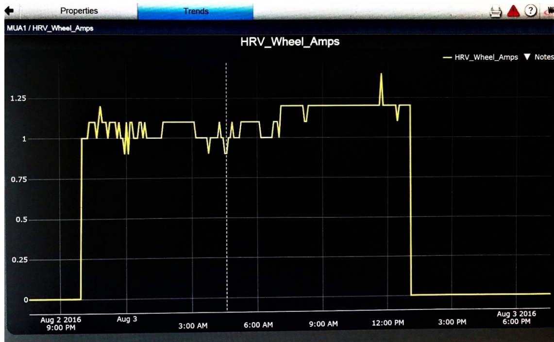
Figure 4.39: Trendlog Graph of Thermal Wheel Amps during August 2016
