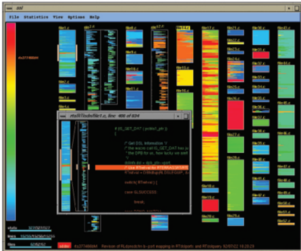
Figure 2.1. Seesoft [1]. Files are displayed as rectangles and the lines of the file are displayed as pixels, with the color of the pixel indicating metrics about the line. In this example, the color of the line represents its age.
