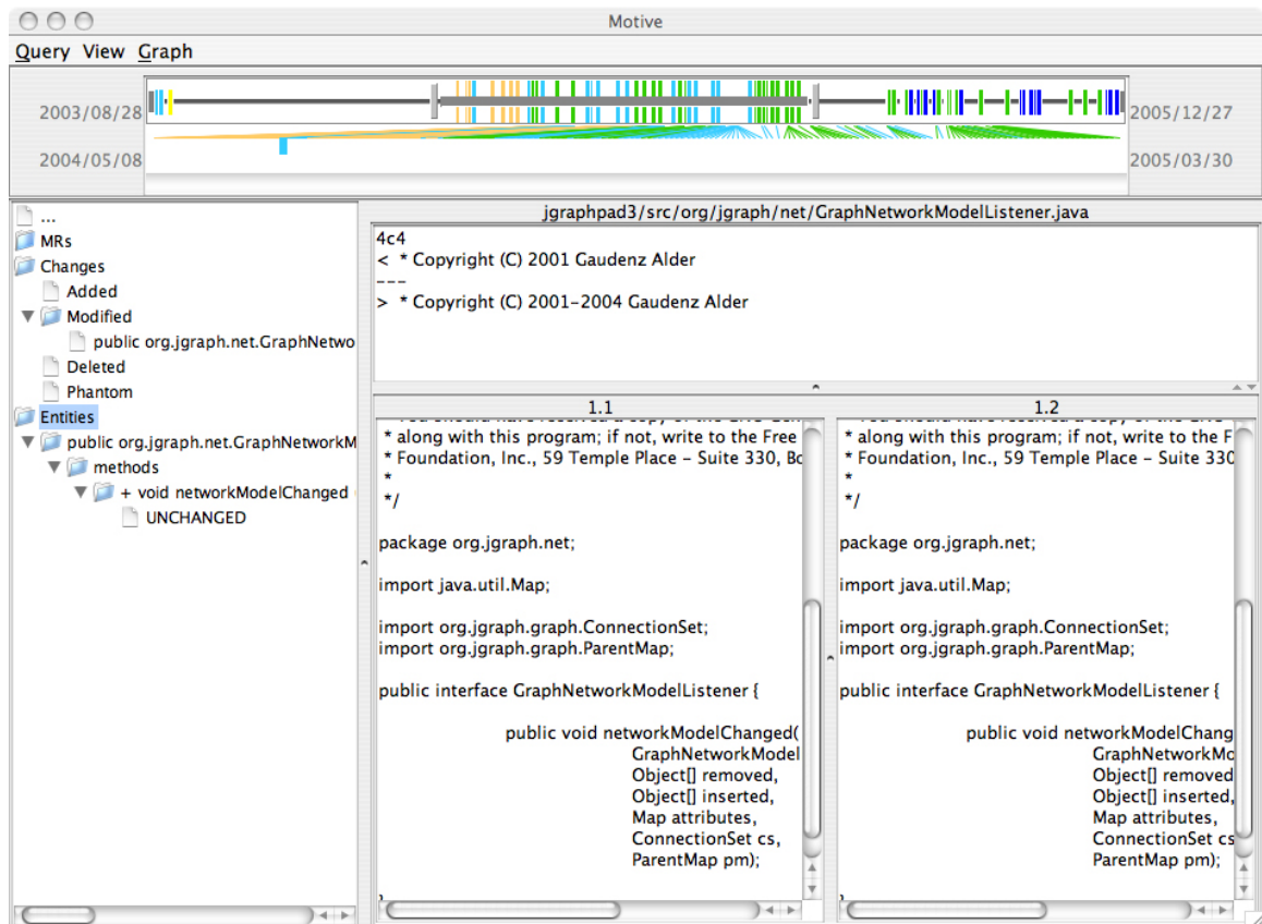
Figure 4.17. A Text View showing the changes from 2004/05/08 - 2005/03/30 to the org.jgraph.net.GraphNetworkModelListener interface. The lower portion of the Text View shows the text of the earliest file revision in the change-set on the left, and the latest on the right. The upper portion shows the output of running diff to compare each file revision in the change-set with the previous revision.
