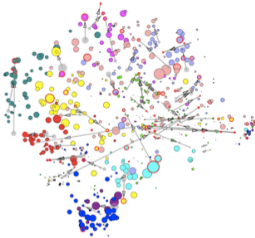
Figure 2.6. An evolutionary storyboard panel for PostgreSQL [2]. Nodes represent files, with the position of the nodes indicating what files were changed together. The arrows show the change in node position from one panel to another. The color of the node represents the subsystem the node belongs to.
