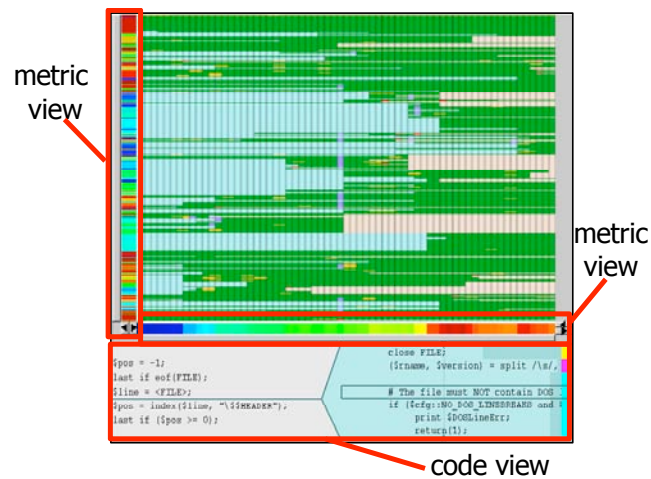
Figure 2.2. CVSScan [42]. CVSScan integrates a line-based view, two metric views, and two text views (indicated in the diagram as the code view).
