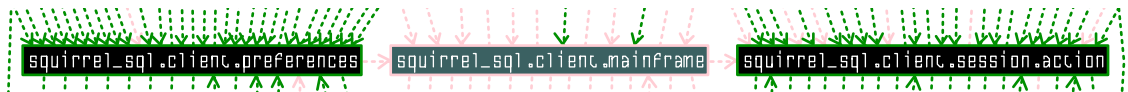
Figure 5.19. A highlight of three packages of SquirrelSQL, shaded according to the number of times they have been modified. The darker the background color of the package, the more MRs have affected the package.
