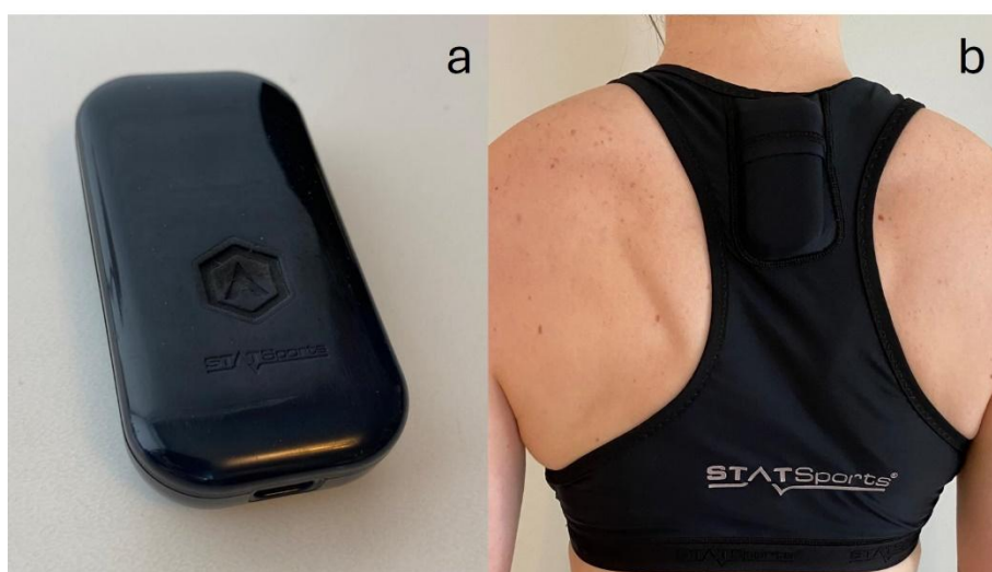
Figure 4.1: (a) GNSS monitor used in data collection and (b) GNSS monitor in vest worn by athlete.
