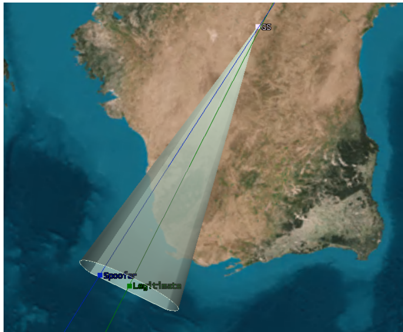
Figure 6.2: The trajectories for l and s within the GS receive antenna HPBW.
