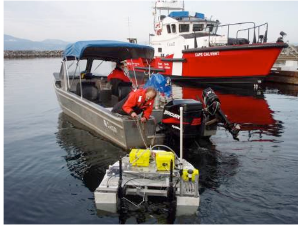
Figure 25. The microlayer sampler being towed from the dock and into Saanich Inlet for sea trials and sensor evaluations.
