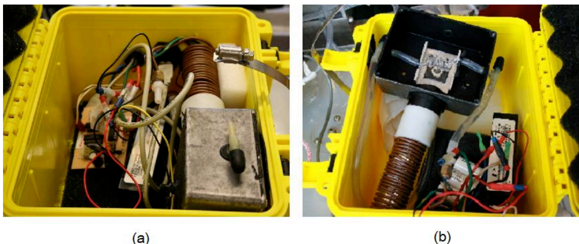
Figure 11. (a) Photograph showing the interior of the housing for the fluorescence spectrometer. Electronics and a box for lighting the sample solution are also shown. (b) The interior of the black box where the water is excited by a Mercury lamp can be seen. Sample water is pumped into the yellow housing and flows around the Mercury lamp, the light source, to cool the lamp after being pumped through the black box.
