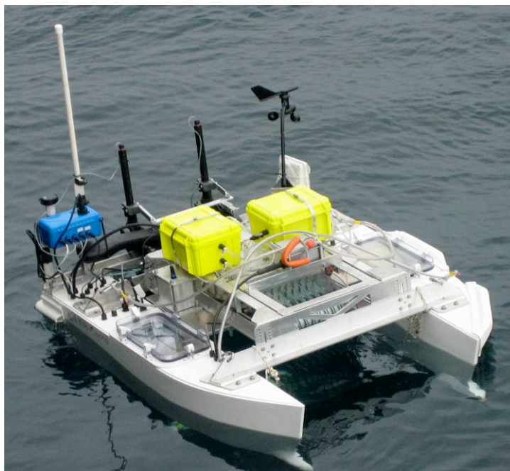
Figure 7. Photograph of the radio controlled vessel with rotating disk microlayer sampler.
