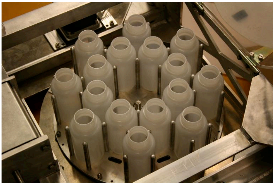
Figure 8. Photograph of sample bottles in the programmable rotating carousel. This carousel can accommodate up to 12 sample bottles, six of which (interior ones) collect microlayer samples collected from the glass disk array, while the other six (exterior ones) collect sublayer water from 1 meter below the surface. The start time of filling and the filling time are completely programmable for each of the six pairs of bottles in the tray.
