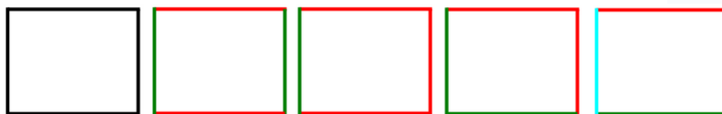
Figure 1.4: Possible configurations in which strokes can be segmented to represent a rectangle with the first rectangle being the raster image and the last one being the most likely way to draw a rectangle by the user.
