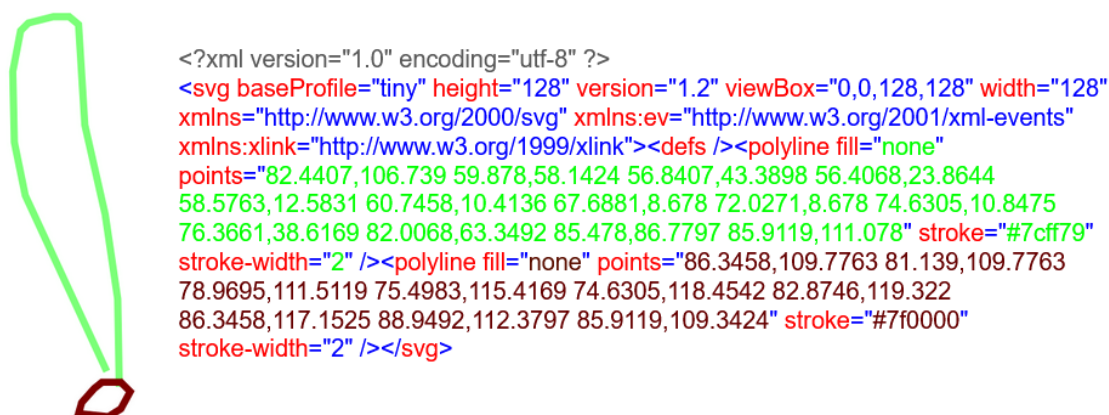
Figure 4.2: Left : SVG image and Right : SVG file format that needs to be converted into PNG format so that it can be used as ground truth for our segmentation model. Each polyline (referred to as vector path in SVG file format) in this file represents a stroke of the line drawing.
