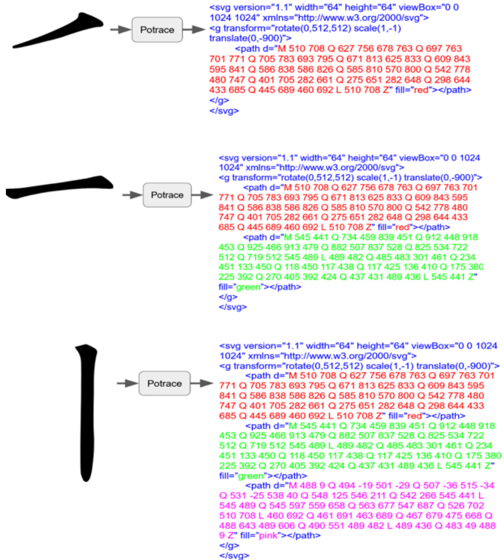
Figure 4.3: Potrace process for a three instance input. The binary mask of each instance is passed through Potrace and the vector path information is added to the SVG document.
