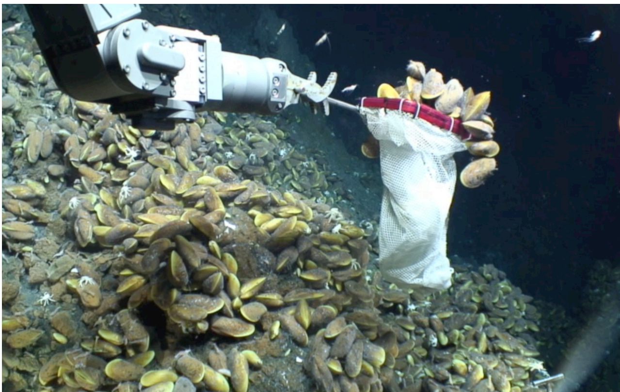
Figure 2.1. ROV Jason II collecting mussels from Golden Lips, NW Eifuku, with scoop net. Scoop net is ~50 cm wide.
