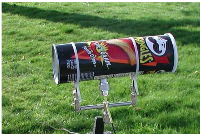
Figure 3-2: The cantenna used for boosting the range of wireless networks.
