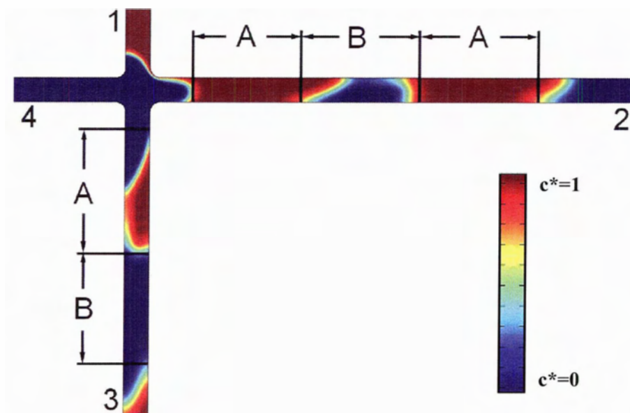
Figure 2.5 Concentration profiles showing the cause of the injection bias for 25 \mu\text{m} channels with 0.05s switch time. In channel 2, Region A is purely solution A but Region B is comprised of both solutions A and B due to the flow lag through the intersection. The result is that the outflow of channel 2 is solution-A-rich and channel 3 is solution-A-poor. [Numerical]
