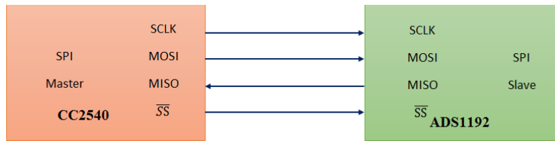
Figure 17: SPI single master and single slave mode
