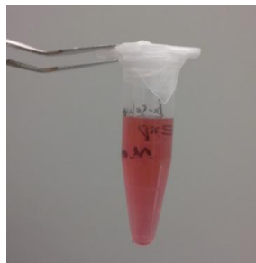
Figure 3.8 Mixture solution of 1, 9-nonanedithiol and colloidal gold particle with ratio N_{thiol/dithiol} : N_{particle} = 1:1 after incubation of 24 h.
