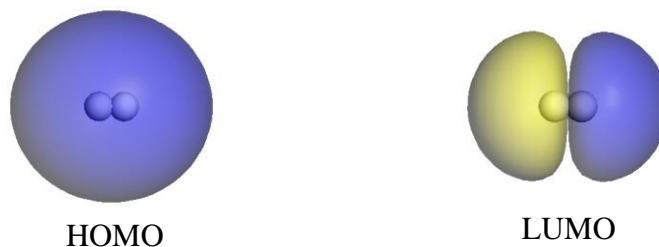
Figure 2.1 HOMO and LUMO of hydrogen molecule. Yellow/blue color represents positive/negative value of wave function. Value of the isosurface is 0.003.
