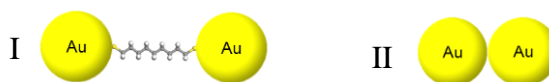
Figure 3.24 I. Particles bridged by one single molecule; II. Particles in direct contact.
