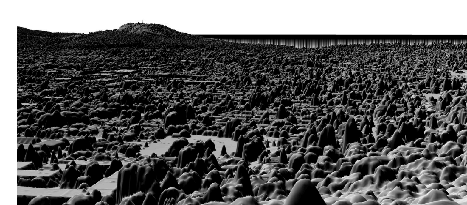
Virtual images were created using a 1m digital surface model (DSM) and user-provided camera parameters. Classified masks were aligned to the corresponding virtual photographs using four control points per image
