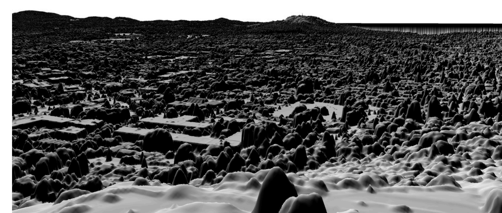
Virtual images were created using a 1m digital surface model (DSM) and user-provided camera parameters. Classified masks were aligned to the corresponding virtual photographs using four control points per image
