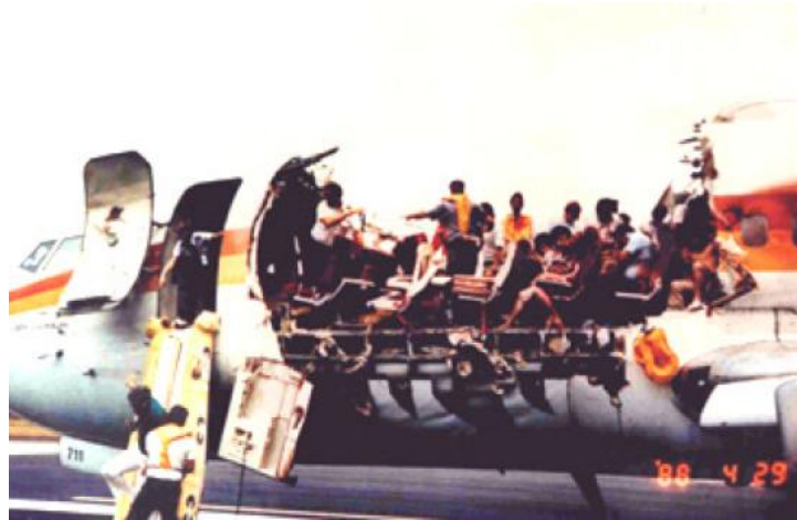
Figure 1.1: Aloha Airlines Boeing 737-297 (tail #N73711), flight 243, Hilo to Honolulu, Hawaii, landed on Kahului Airport on Maui, April 28, 1988 - multi-site fatigue-corrosion crack damage in non predicted locations in the fuselage skin panel joints – ageing structure aggravated by commuting service with frequent short flights with take-off, compression-decompression cycles and landings [1].
