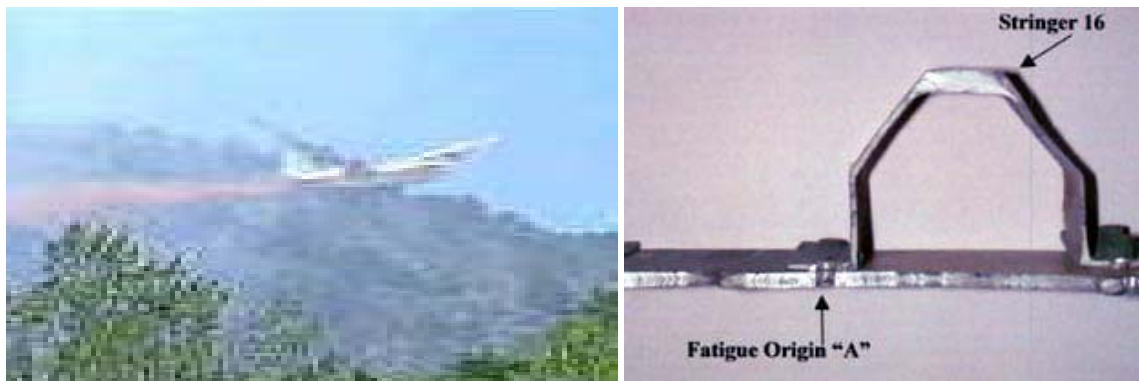
Figure 1.3: Hawkins & Powers Aviation C-130A fire fighter (Tail#N130HP), Walker, California, June 17, 2002 - fatigue cracks in the wing structure [3].
