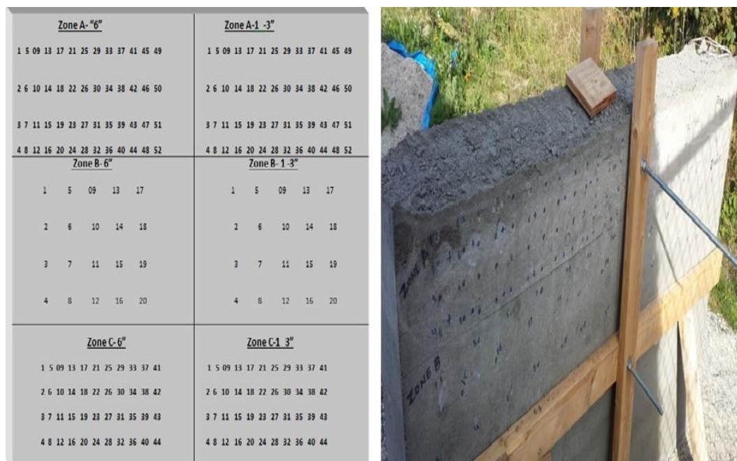
Figure 8 - Rammed earth wall reading points: a) schematic plan and b) actual wall specimen
