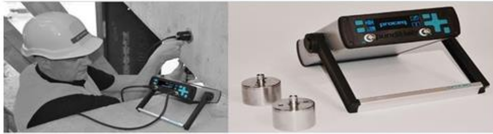
Figure 11 - UPV equipment and quality ranges [8]
