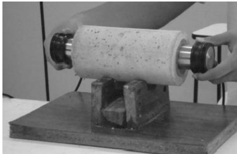
Figure 14 - Application of the UPV method to cylinders [10]
