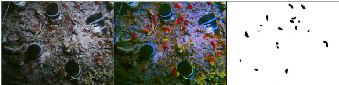
Figure 8: A) Image representing the large field of view with all 25 temperature loggers visible. In the left circle is a Branchinotogluma sp. individual and in the right circle a Lepidonotopodium piscesae individual. B) Image analysis process; the original image (left) obtained from the small field of view, the same image (center) following brightness, contrast and saturation correction and the resulting binary image (right) where black dots represent Branchinotogluma sp. individuals.
