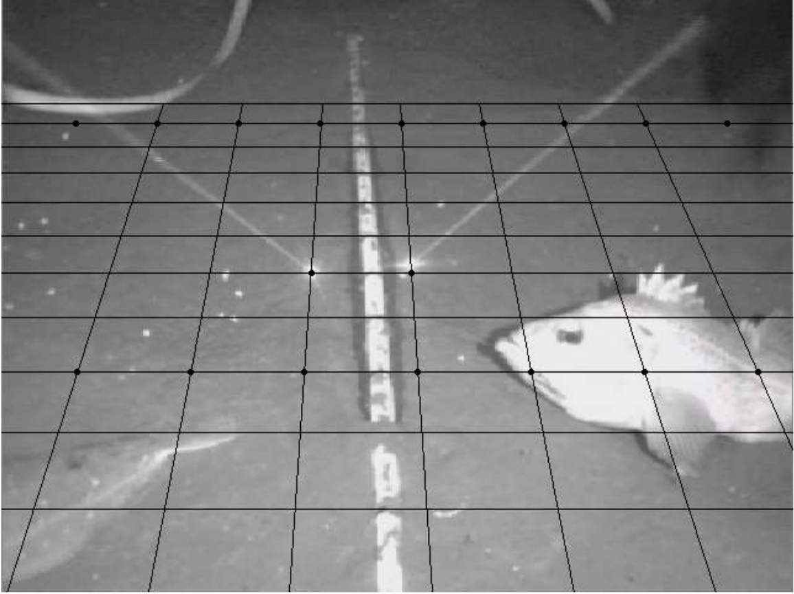
Figure 2: Perspective grid for the Axis site with a tilt = 30. The scaling ruler with 10 cm increment is visible in the center of the image and the laser beams are separated by 10 cm. Hence, each square represents 100 \text{ cm}^2 on the seafloor.
