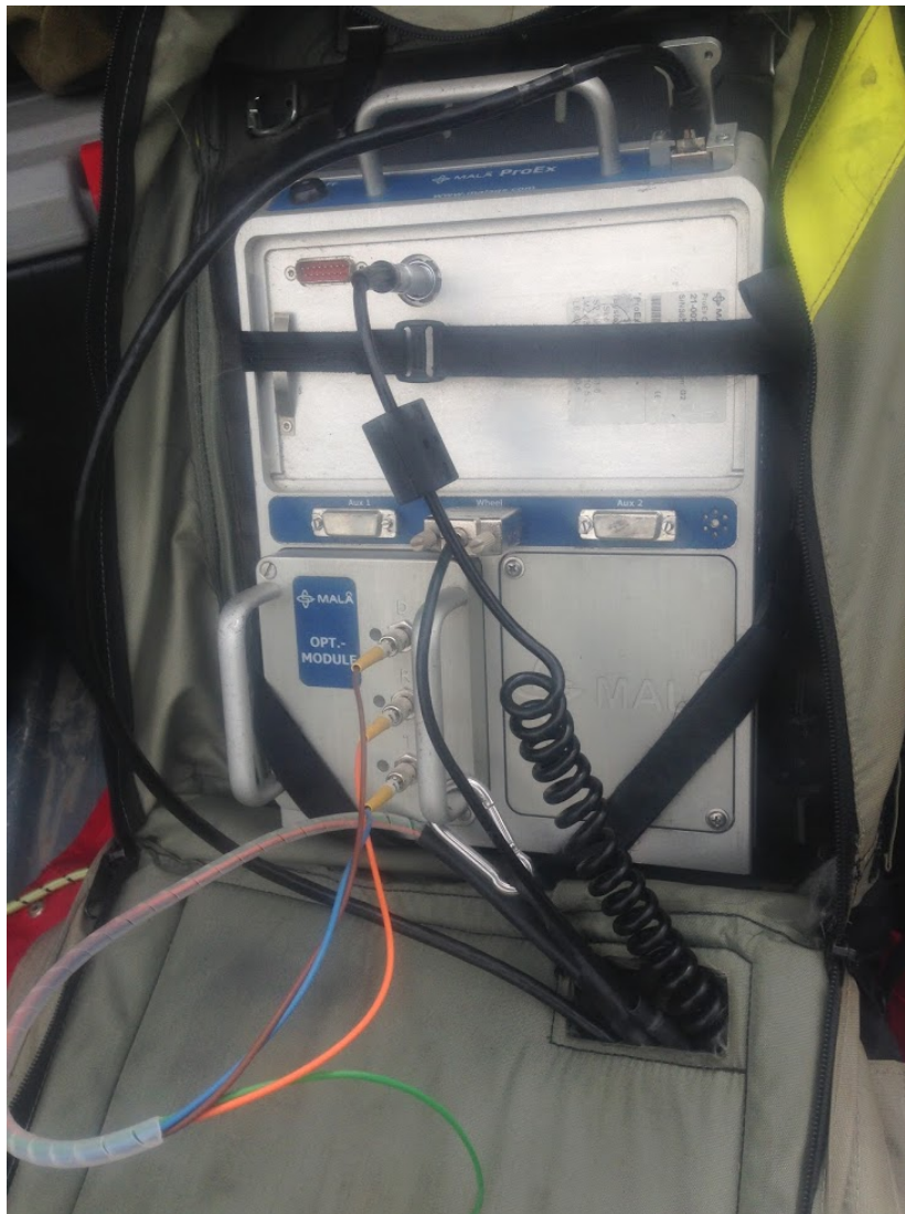
Figure 9.6 MALÅ ProEx System with Optical Module, photo by Wm.Shulba
