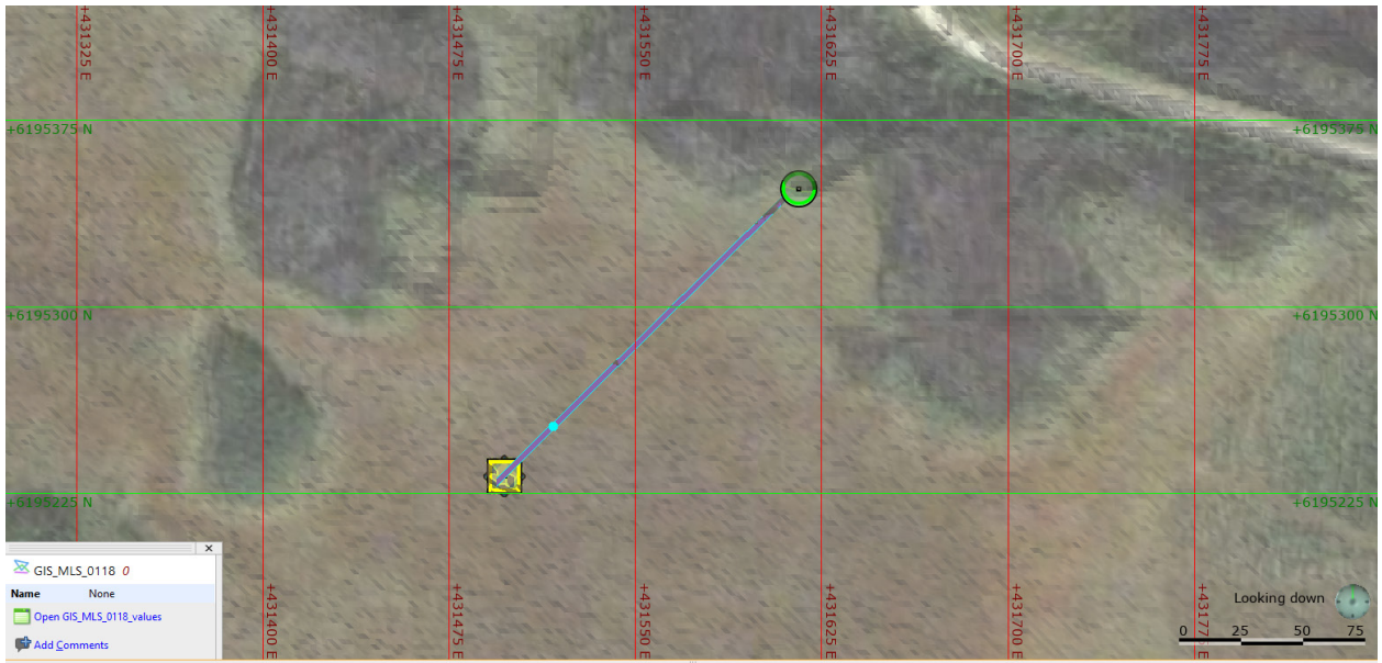
Figure 4.43 Plan view selecting location markers for import of GPR cross-section.
