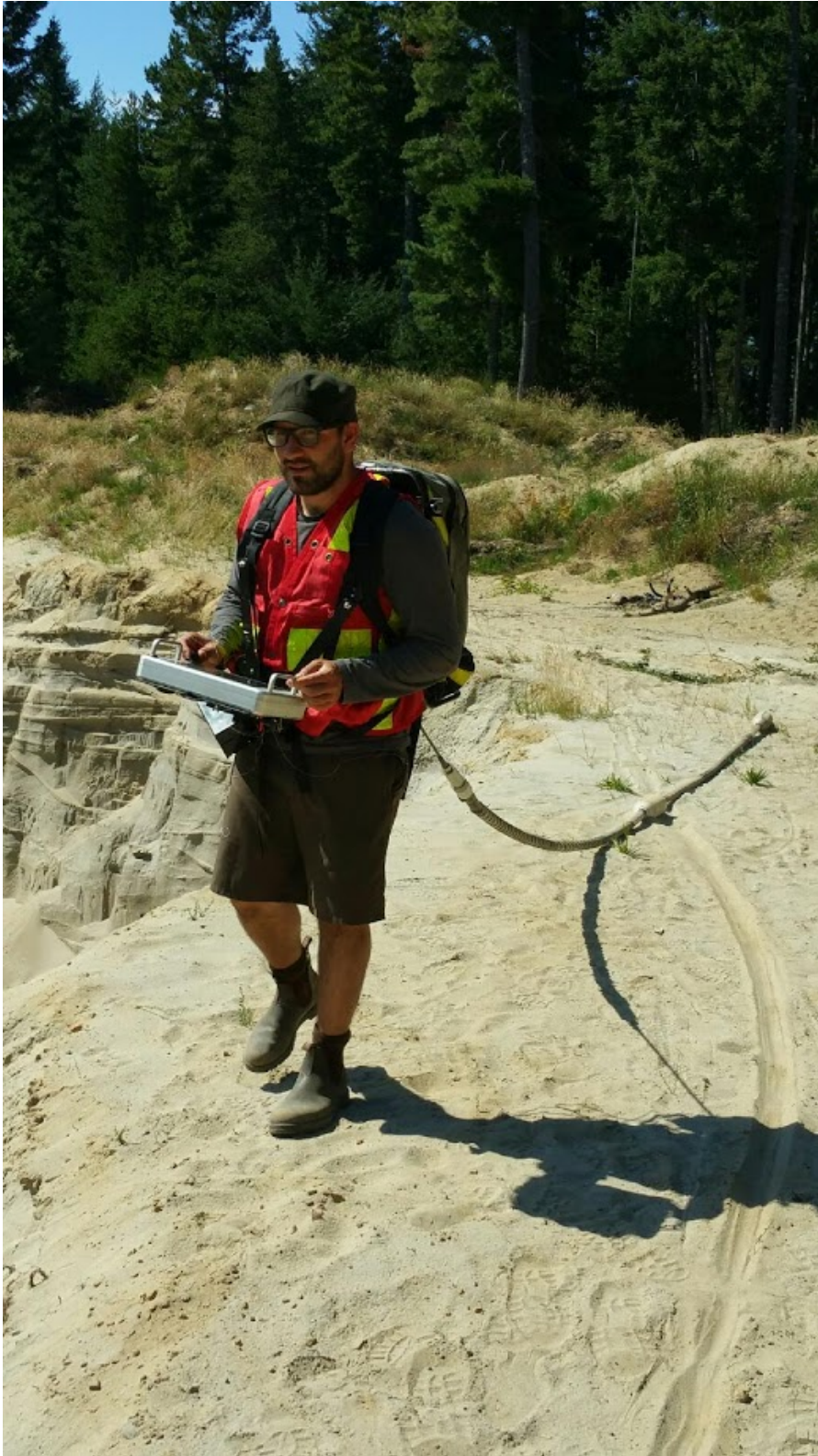
Figure 9.3 MALÅ RTA Antenna at a Sedimentary Sequence near Oyster River on Vancouver Island.
