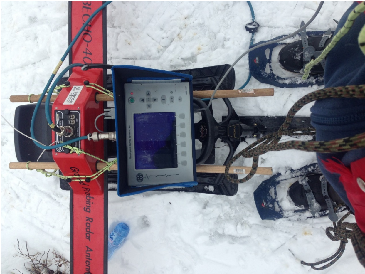
Figure 9.9 GSSI 3000 Controller with Subecho40 GPR Antenna
