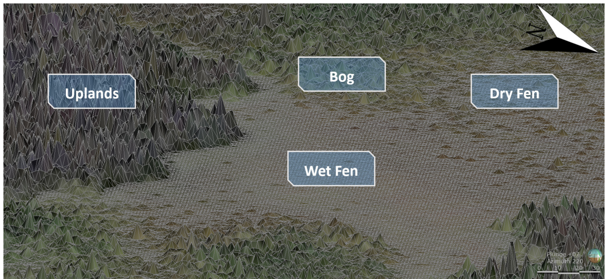
Figure 5.1 First reflection DEM mesh with triangulation showing ecological units from microtopographic texture
