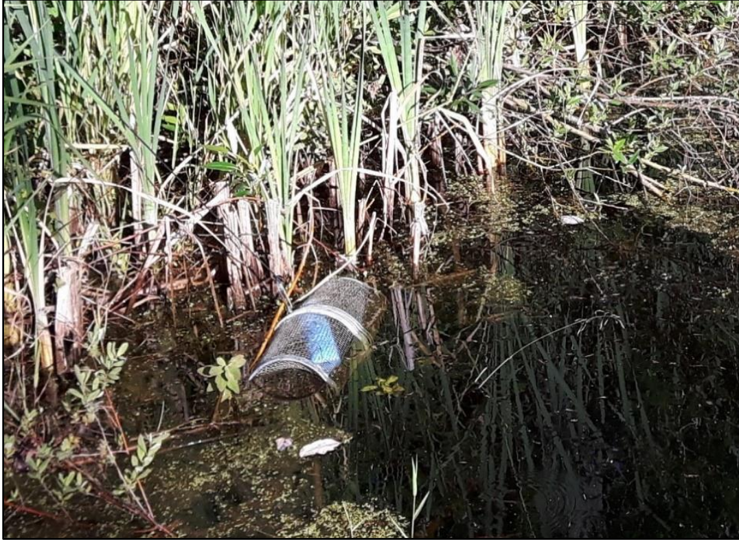
Figure 2.1 Deployed minnow trap oriented parallel to littoral vegetation and kept partly submerged with foam float.
