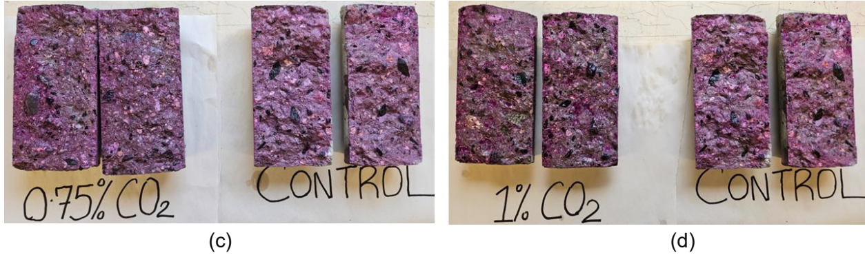
Figure 4.11 Comparison of CO 2 -sequestered concrete and control samples sprayed with phenolphthalein: (a) Control vs. 0.25% CO 2 , (b) Control vs. 0.5% CO 2 , (c) Control vs. 0.75% CO 2 , and (d) Control vs. 1.00% CO 2
