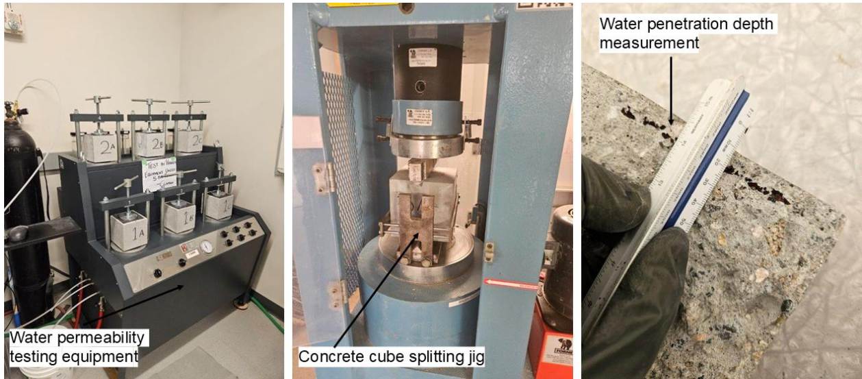
(a) (b) (c) Figure A.5 (a) Water permeability testing setup, (b) Concrete cube splitting jig and (c) Water penetration depth measurement
