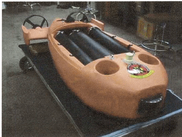
Fig. 6. Cetus hybrid AUV with two aft thrusters and two vertical tunnel thrusters in the nose [7].
