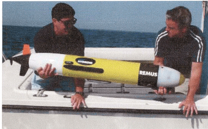
Fig. 4. The REMUS AUV being manually deployed from a small vessel [4].
