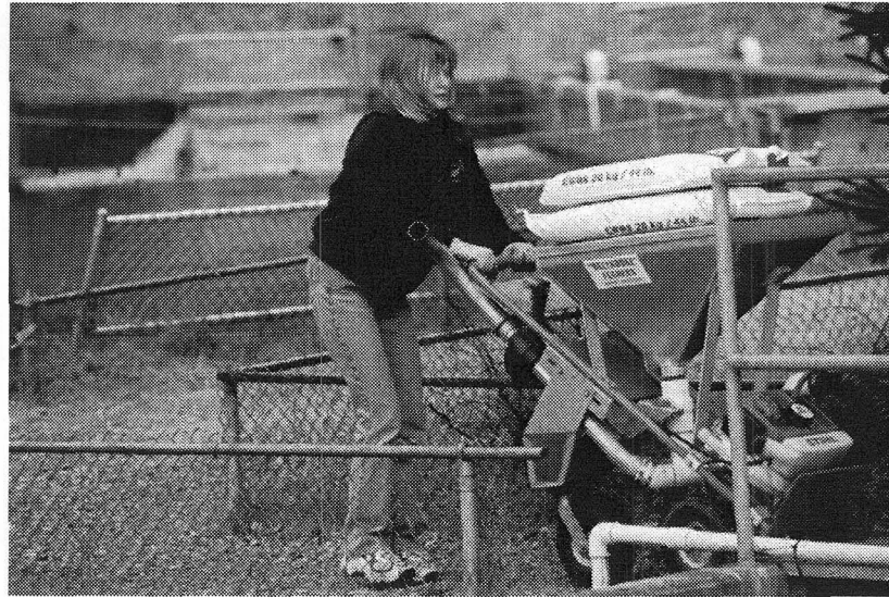
Figure 3.1. The mechanical fish feeder that was converted from a commercial leaf-blower. It is seen here being towed into position next to a pond by a fish culturist. The machine, built by a fish culturist from a nearby hatchery, was exchanged for some excess feed in Shallow River. Photograph used with permission from Wolff-Michael Roth.
