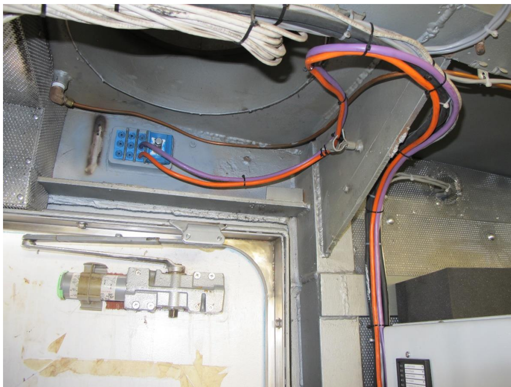
Figure A-11: Wire Routing through Rextec Fireproof/Waterproof Bulkhead Pass-Throughs
