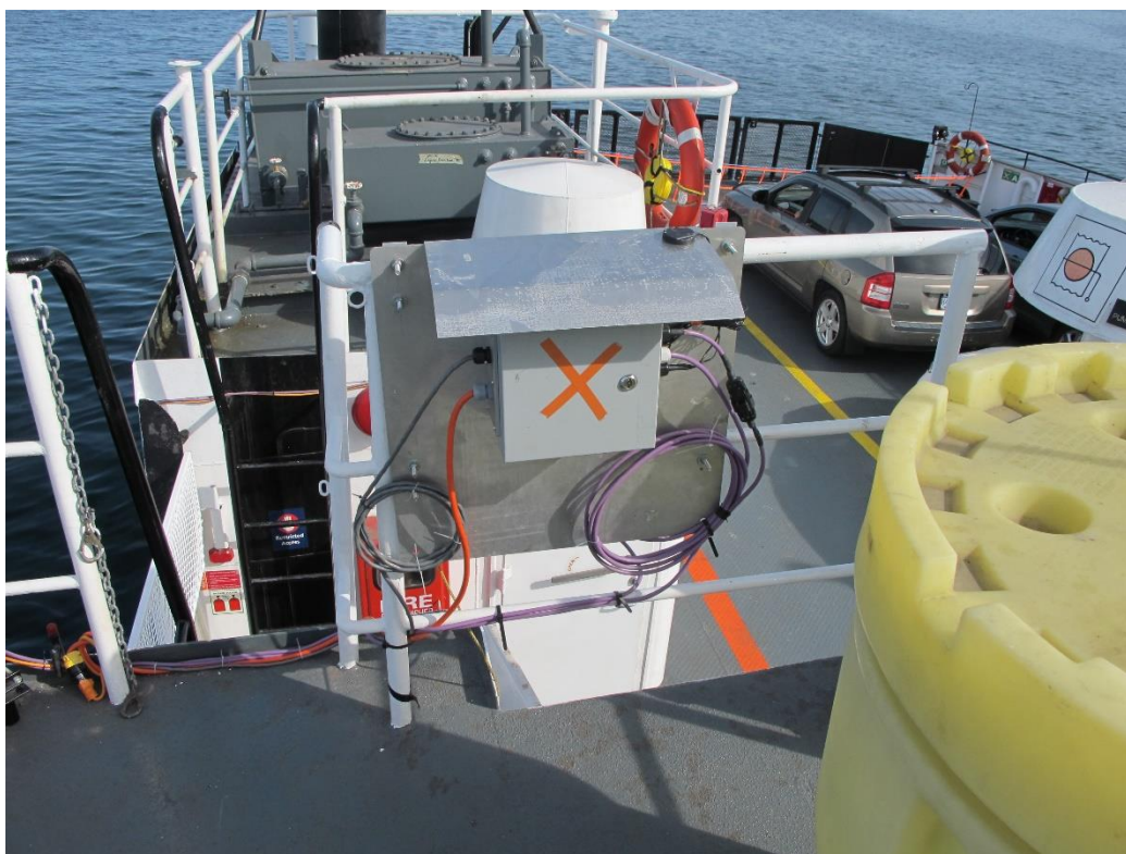
Figure A-8: GPS Unit and CAN Data Logger Installation
