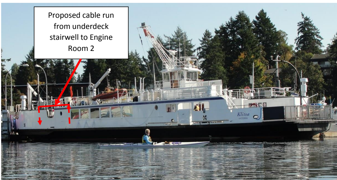
Figure 21: Proposed Outdoor Wiring Route between Lower Deck Stairwell, GPS Location, and Engine Room 2
