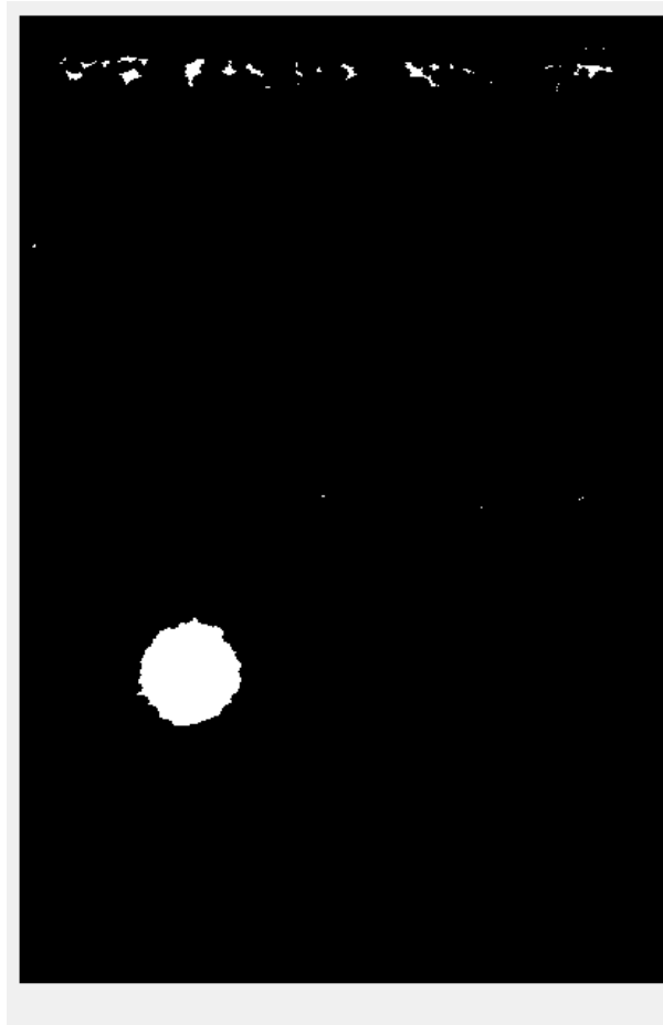
Figure 2.4: Binary image after filling holes, clearing borders and image complement.
