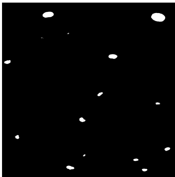
Figure A-2 Image of selected area in NaDC-CB6 gel tagged with rhodamine 6G ( 2 \mu\text{M} ) at CB[6]/NaDC ratio of 0.05 after adjusting the threshold.
