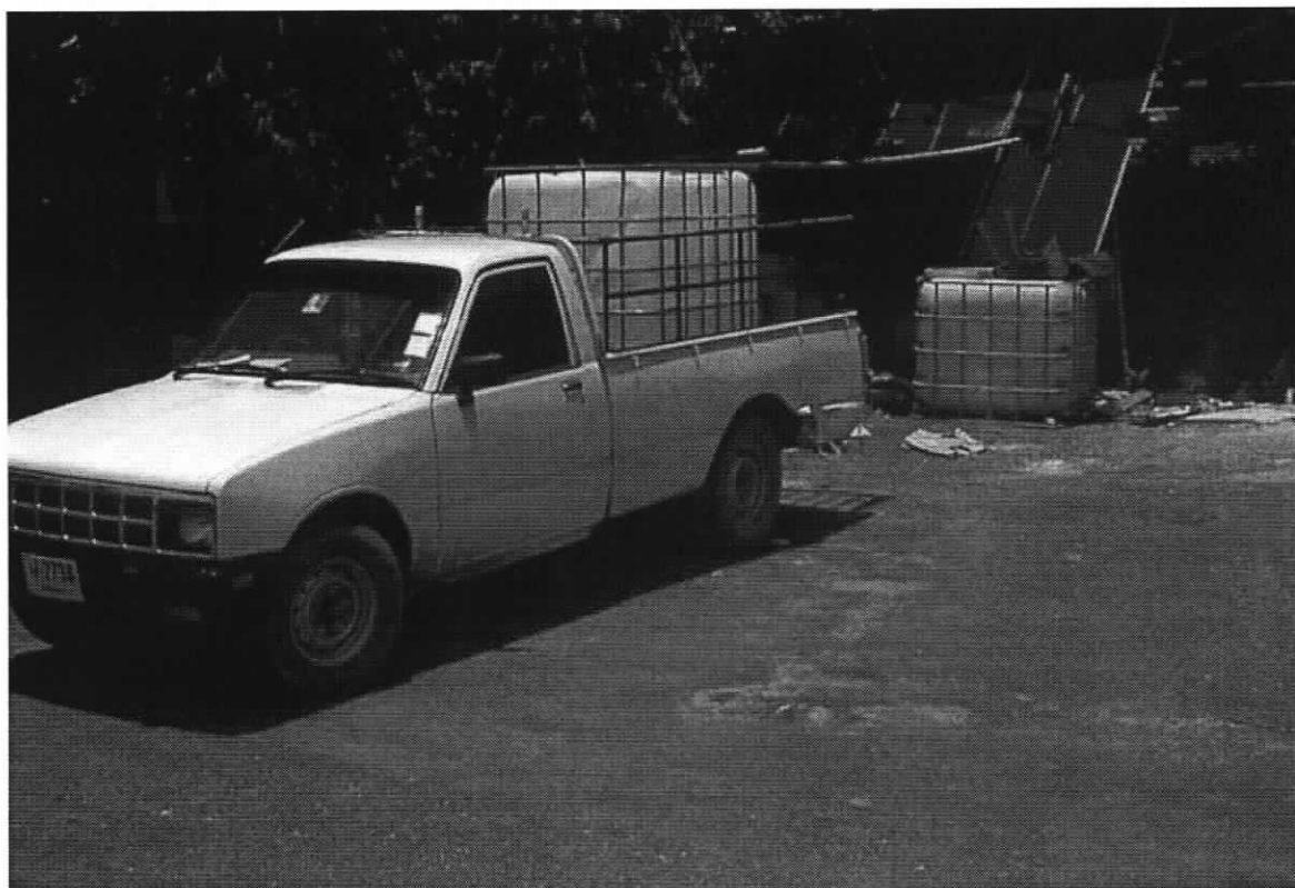
Figure 5.8 Small Pickup Truck with Tank Used for Local Saline Water Delivery to Low-Salinity Shrimp Farms
