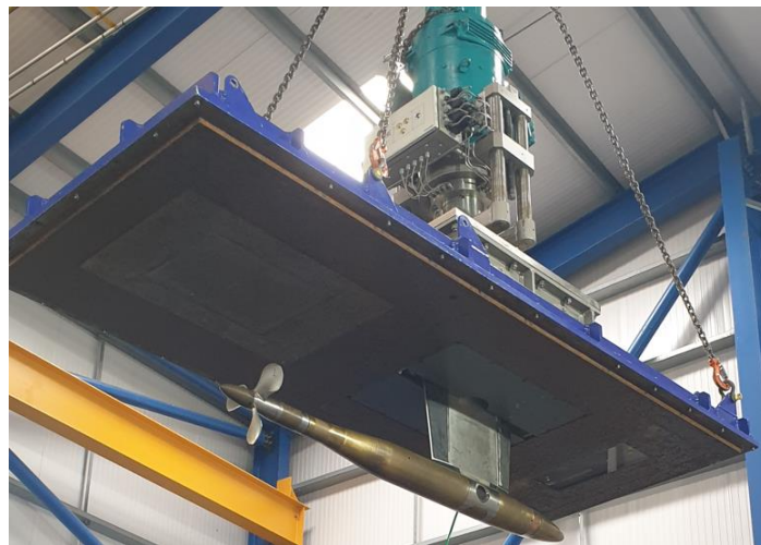
Figure 2. Kempf & Remmers H45 torpedo-shaped fitting with 0 degrees of skewness tidal turbine mounted.
