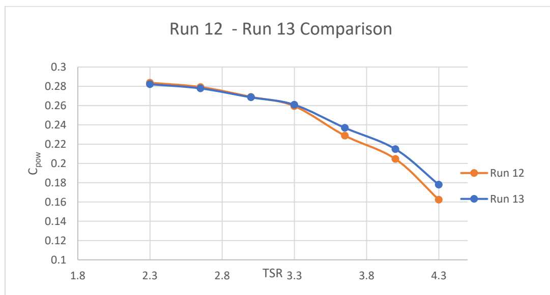
Figure 7. Test run 12 and test run 13, C_{pow} vs. TSR comparison.
