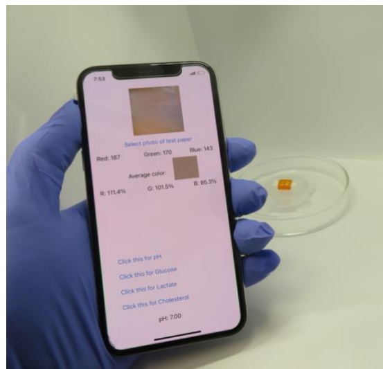
Figure 16: The applications UI displays average RGB values (from 0-255), image of the average color, average RGB percentage values and detected biomarker values.
