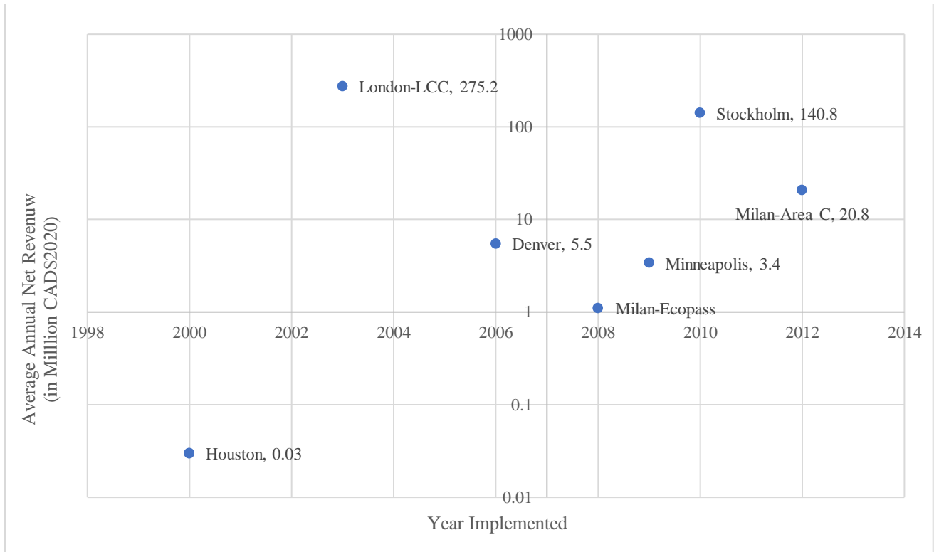
Figure 18: Average annual net revenue of congestion pricing systems by jurisdiction and system implementation year. Net revenue has been brought a consistent value in CAD$2020.
