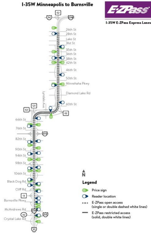
Figure 11: Map of the I-35W Express Lanes. Green tags indicate pricing signage. Purple tags indicate tolling gantries (Minnesota Dept of Transportation, n.d.-a).
