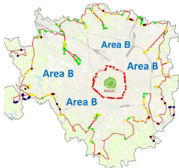
Figure 13: Map of Milan's Area B. Single red line indicates zone's boundary. Coloured dots indicate electronic tolling gate - different colours indicate the different phases in which gates were installed (Municipality of Milan & Mobility and Environment Department, 2019).
