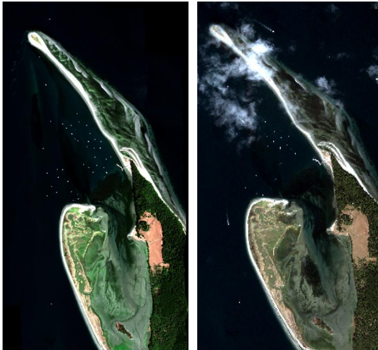
Figure 4.1 RGB composite of the (a) hyperspectral AISA image (R = 650, G = 550, B = 450nm) (2 x 2 m resolution) and (b) multispectral IKONOS image (R = 665 nm, G = 550nm, B = 480nm) (4 x 4 m resolution).
