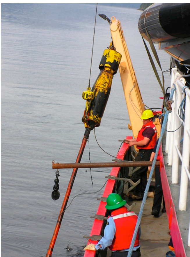
Figure 3.4 : Left- Piston coring aboard CCGS Vector (photograph taken in April, 2009). Right- Piston core assembly including piston core barrel, trip arm assembly, and pilot gravity core (from Buckley et al., 1994).
