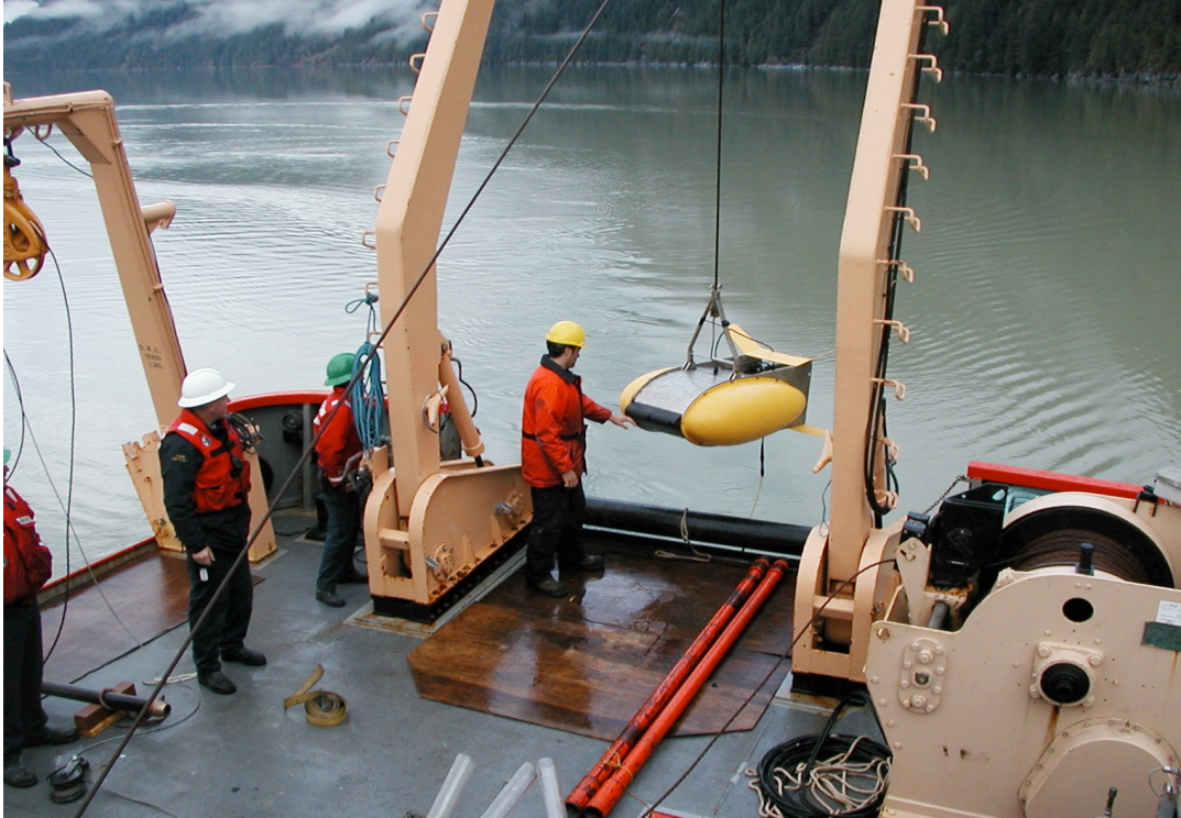
Figure 3.1 : A deep-tow Hunttec seismic system as it goes in the water in preparation for surveying. Picture taken aboard the CCGS Vector (November, 2007).
