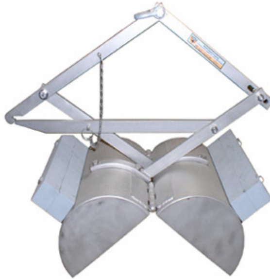
Figure 3.3 : Petersen Grab sampler operates on a lever system whereby the jaws release under its own weight and close upon sediments on the seafloor.
