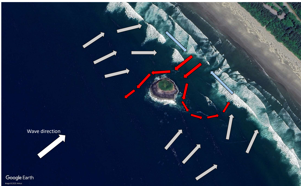
Figure 4.5: Rip current flow at Lovekin Rock as observed on 8 August 2025.
