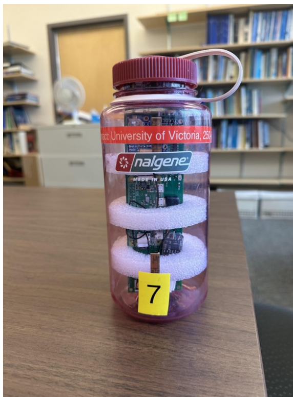
Figure 2.12: Surf zone drifter modified from the design of Rainville et al (2023).
