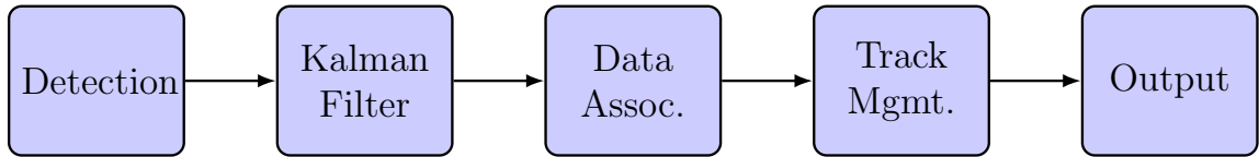
Figure 2.4: Diagram of the SORT (Simple Online and Realtime Tracking) algorithm, illustrating its streamlined process for multi-object tracking. The figure outlines the key phases of detection, state prediction with a Kalman Filter, data association using the Hungarian algorithm, and track management.
