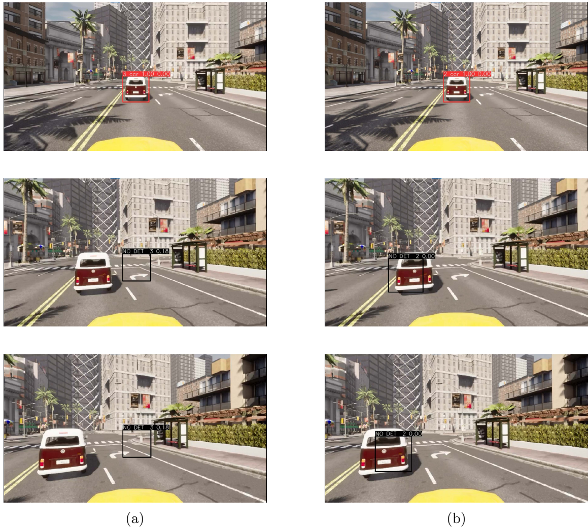
Figure 4.1: In this scenario, the object detection is missed, leading to a failure in predicting the location of the object during lane-changing for Vanilla ByteTrack (a). ByteTrack + EMAP (b) significantly improves the prediction, successfully tracking the object in the next two frames.
