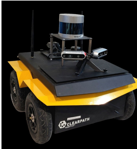
Figure 2.3: The Jackal UGV equipped with a Velodyne VLP-16 LiDAR, two RGB-D cameras, wheel encoders, and an IMU, demonstrating its comprehensive sensor suite for advanced robotic applications.
