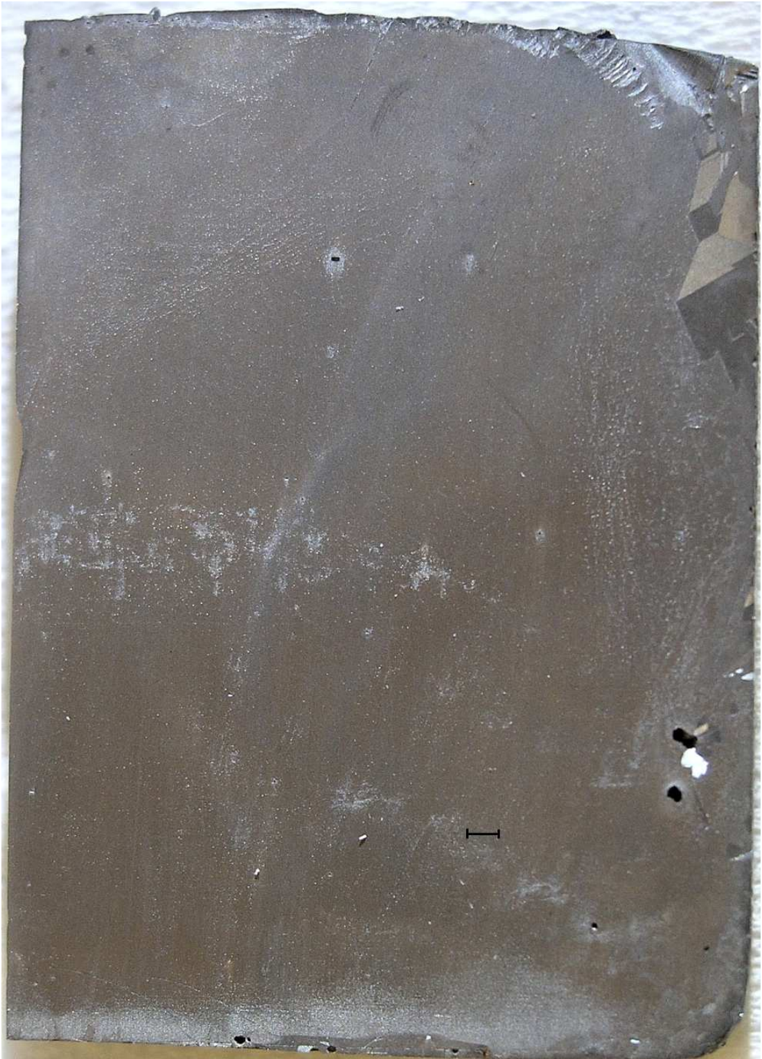
Figure 6.5: Section of Experiment 12 after polishing and etching. Scale mark is 1 mm wide.
