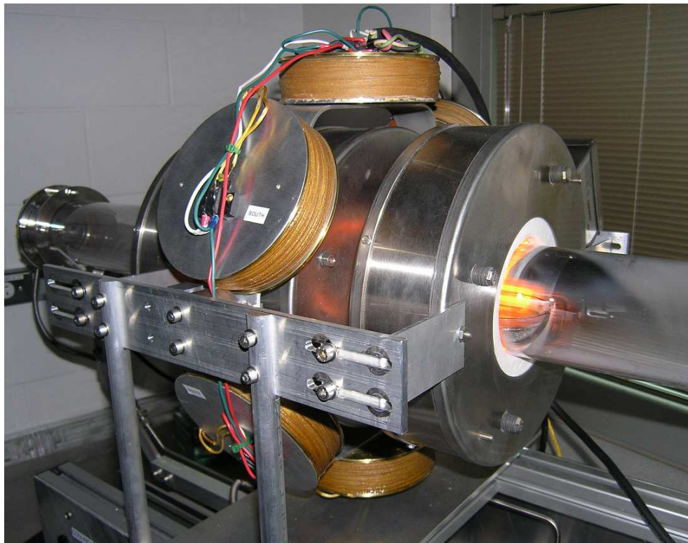
Figure 3.5: The zone refining apparatus with RMF coils installed on the middle heater
