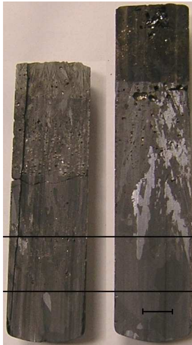
Figure 4.1: Ingots from experiments 8 and 12. CdTe grown from the bottom at 15, 65 and 70 mm/day. Black lines indicate approximate locations of changes in growth velocity. Scale mark is 10 mm wide.
