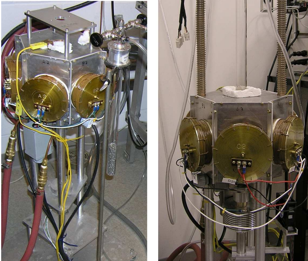
Figure 5.1: The THM furnace before and after modification for GaSb single crystal growth
