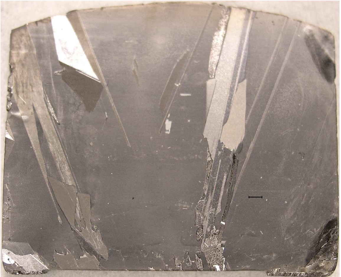
Figure 6.2: Section of Experiment 10 after polishing and etching. Scale mark is 1 mm wide.
